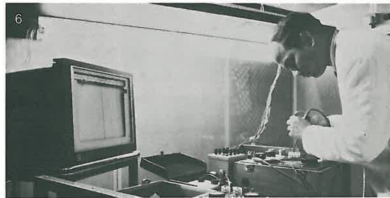
Some items in the exhaustive testing programme at the Enfield laboratories. Here can be seen (1 and 2) the fitting being installed in the polar-curve photometer and the integrator to measure its light distribution and light-output ratio; (3). An enlarged shadow, check of the acrylic prismatic controller; (4 & 5) heat test on the lampholder and 'finger test' on all live parts. In tests for thermal safety thermo-couples are connected to all 'hot spots' (6) and a needle-flame test (7) ensures non flammability of the glass filled nylon plastic mains terminal socket.
