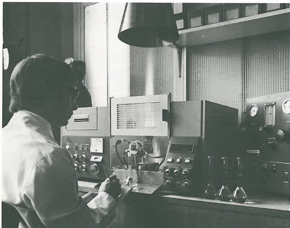
The Atomic Absorption Spectrophotometer. This analyses the chemical composition of phosphors.
