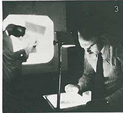
Some items in the exhaustive testing programme at the Enfield laboratories. Here can be seen (1 and 2) the fitting being installed in the polar-curve photometer and the integrator to measure its light distribution and light-output ratio; (3). An enlarged shadow, check of the acrylic prismatic controller; (4 & 5) heat test on the lampholder and 'finger test' on all live parts. In tests for thermal safety thermo-couples are connected to all 'hot spots' (6) and a needle-flame test (7) ensures non flammability of the glass filled nylon plastic mains terminal socket.
