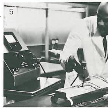
Some items in the exhaustive testing programme at the Enfield laboratories. Here can be seen (1 and 2) the fitting being installed in the polar-curve photometer and the integrator to measure its light distribution and light-output ratio; (3). An enlarged shadow, check of the acrylic prismatic controller; (4 & 5) heat test on the lampholder and 'finger test' on all live parts. In tests for thermal safety thermo-couples are connected to all 'hot spots' (6) and a needle-flame test (7) ensures non flammability of the glass filled nylon plastic mains terminal socket.
